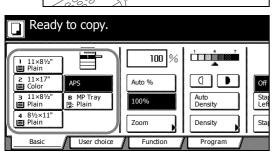
**3** Confirm that [APS] is selected. In this mode, paper that matches the size of the originals will be selected automatically. To change the paper size, press the desired paper size to select the paper source.
